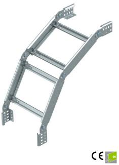
90° adjustable vertical bend, for cable ladders with medium-duty rung (VS) and a side height of 60 mm. The fitting is shipped in an unmounted state including adjustable connectors and
