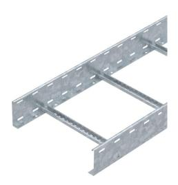
Cable ladder with 110 mm side height with riveted C profile rungs which are open in an upwards direction. Rolled side rail for reinforcement and as edge protection. Fastening to the bracket takes place using hold-down clamps, type LKS 60/4. The slot dimension of the rung is 16.5 mm and the appropriate clamp clip is type 2056
