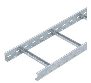
Cable ladder with perforated side rail of side height 60 mm with riveted C profile frames, open in an upwards direction (VS version).
