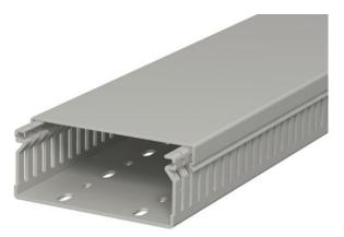
Wiring duct, incl. cover and base perforation, for horizontal and vertical routing of electrical cables in the switchgear cabinet. Designed as a metric duct. The nominal dimension of the system size corresponds to the internal dimension of the duct. Retainers are broken out without tools. The flush-floor routing of cables is possible through predetermined break points. Tested to DIN EN 50085-2-3. Special lengths on request.
