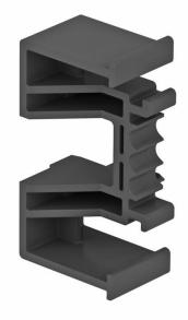
Adapter for the installation of accessory mounting boxes of the 71GD... series in WDK wall and ceiling trunking. The use of accessory mounting boxes, type 71GD8 and 71GD9, permit standardised installation of Modul 45 devices. Devices can be installed in the trunking heights 110, 130 and 150 mm. Combined with device covers of the AR45-... series, finished cover sections of the OT GE ... series can cover the switching and connection devices.
