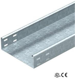
MKSU 60 = medium-duty cable tray system, unperforated, with a side height of 60 mm. Straight connectors should be ordered in the appropriate quantity. The cable tray has connector perforations on both sides. Magnetic shield insulation without cover 20 dB, with cover 50 dB.
