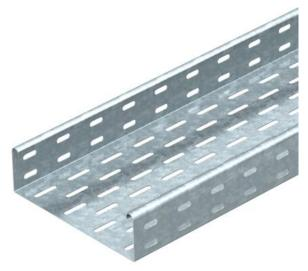
MKS 60 = Medium-duty cable tray system with a side height of 60 mm. The cable tray is fastened to the bracket with bolts, type FRS M6 x 12. The surface coating is a coating created in a single-dip method with extra-high zinc thicknesses
