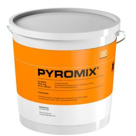
Mortar to create cable and combination insulation in solid walls and ceilings. Suitable for pumping, pressing and for manual installation. Adding approx. 3 litres of water to 10 kg of dry mortar produces about 10 litres of workable compound. For interior application.
