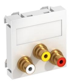
Multimedia support with three cinch connection sockets for audio-video, straight cable outlet, with labelling panel, three cinch sockets (RCA) with soldered connection, colour coding yellow / red / white. Support plate with locking fastening, suitable for horizontal and vertical installation in the system environment.
