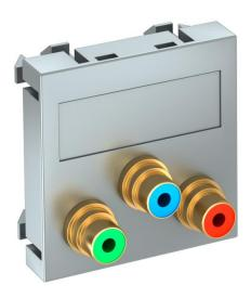
Multimedia support with three cinch connection sockets for component video, straight cable outlet, with labelling panel, three cinch couplings (RCA), socket-socket version, colour coding red/green/blue. Support plate with locking fastening, suitable for horizontal and vertical installation in the system environment.
