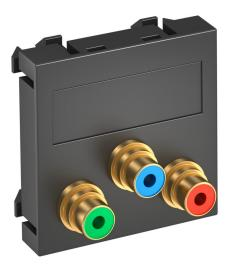
Multimedia support with three cinch connection sockets for component video, straight cable outlet, with labelling panel, three cinch sockets (RCA) with soldered connection, colour coding red / green / blue. Support plate with locking fastening, suitable for horizontal and vertical installation in the system environment.
