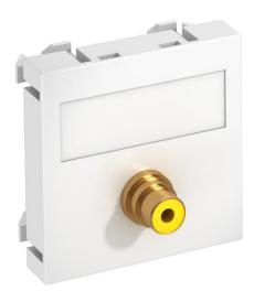
Multimedia support with one cinch connection socket for composite video, straight cable outlet, with labelling panel, cinch socket (RCA) with soldered connection, colour coding yellow. Support plate with locking fastening, suitable for horizontal and vertical installation in the system environment.
