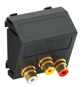
Multimedia support with three cinch connection sockets for audio/video, slanting cable outlet, with labelling panel, three cinch couplings (RCA), socket-socket version, colour coding yellow/red/white. Support plate with locking fastening, suitable for horizontal and vertical installation in the system environment.
