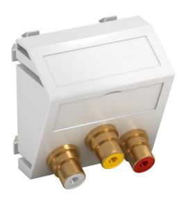
Multimedia support with three cinch connection sockets for audio/video, slanting cable outlet, with labelling panel, three cinch sockets (RCA) with soldered connection, colour coding yellow / red / white. Support plate with locking fastening, suitable for horizontal and vertical installation in the system environment.
