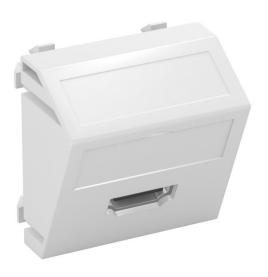
Multimedia support with one HDMI connection socket, slanting cable outlet, with labelling panel, HDMI socket with screw connection. Support plate with locking fastening, suitable for horizontal and vertical installation in the system environment
