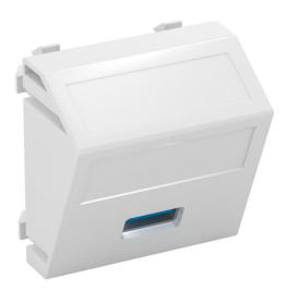
Multimedia support with one USB 3.0 connection socket, slanting cable outlet, with labelling panel, USB 3.0 type A socket with screw connection. Support plate with locking fastening, suitable for horizontal and vertical installation in the system environment.
