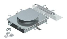
Ready-to-mount trunking extension unit with a device installation lid for the installation of a flush-mount unit of nominal size R9, consisting of the trunking base (floor trough with side and floor covering contact profiles), trunking lid with blank mounting opening and a flushfloor end cover. The scope of delivery contains 3 height-adjustable fixing brackets, 3 screed anchors, 1 lid butt support and 1 construction set for 90° angle
