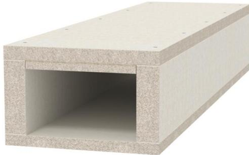
Fire protection duct made of water and frost-resistant fibreglass lightweight concrete of material class A1 according to EN 13501-1 for fireproof routing of cables in escape and rescue routes. EI60 classification as installation duct according to EN 13501-2 on the basis of tests according to EN 1366-5. When there is an internal fire load (cable fire), the duct prevents the spread of fire from one fire section to another.
