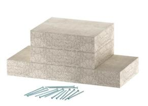
Wall connection collar for PYROLINE® Con D El60 fire protection duct, type PLCD D060810 consisting of fibreglass light concrete, which is resistant to water and frost, for mounting on the fire protection duct in the area of wall and ceiling connections and wall and ceiling penetrations. Consists of 3 single plates (width 100 mm, depth 30 mm). Including countersunk head screws.
