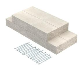
Wall connection collar for PYROLINE® Con S El90 fire protection duct, type PLCS D090810, consisting of fibreglass light concrete, which is resistant to water and frost, for mounting on the fire protection duct in the area of wall connections and wall penetrations. Consists of 4 single plates (width 50 mm, depth 30 mm).
