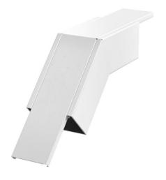
45° vertical bend, falling version, with intumescent fire protection mesh for PY-ROLINE® Rapid PLM installation duct. Suitable for direct wall and ceiling mounting, mounting below system floors and on support systems. Tool-free joint mounting with PLM SI joint connector. The cover is snapped on without tools, allowing rapid inspection and retroassignment. The cover overhang allows offset cover mounting for continuous equipotential bonding of the entire duct section.
