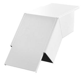
45° vertical bend, falling version, with intumescent fire protection mesh for PY-ROLINE® Rapid PLM installation duct. Suitable for direct wall and ceiling mounting, mounting below system floors and on support systems. Tool-free joint mounting with PLM SI joint connector. The cover is snapped on without tools, allowing rapid inspection and retroassignment. The cover overhang allows offset cover mounting for continuous equipotential bonding of the entire duct section.
