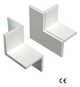
Wall connection collar, 2-sided, with integrated seal for PYROLINE® Rapid PLM installation duct. For mounting in the area of wall and ceiling connections as well as wall penetrations in room corners. Set consisting of 2 opposing components, suitable for ceiling or wall mounting of the installation duct.
