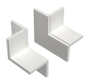
Wall connection collar, 2-sided, with integrated seal for PYROLINE® Rapid PLM installation duct. For mounting in the area of wall and ceiling connections as well as wall penetrations in room corners. Set consisting of 2 opposing components, suitable for ceiling or wall mounting of the installation duct.
