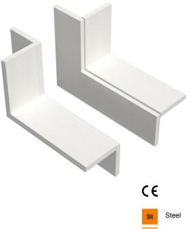
Wall connection collar, 2-sided, with integrated seal for PYROLINE® Rapid PLM installation duct. For mounting in the area of wall and ceiling connections as well as wall penetrations in room corners. Set consisting of 2 opposing components, suitable for ceiling or wall mounting of the installation duct.
