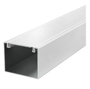
Metal installation duct with intumescent fire protection mesh for fireproof routing of cables. Classified as an installation duct El30, El60 and El90 according to EN 13501-2, tested according to EN 1366-5. The duct prevents the fire spread for the classified period of time, offering protection against the effects of a cable fire.
