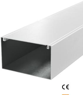
Metal installation duct with intumescent fire protection mesh for fireproof routing of cables. Classified as an installation duct El30, El60 and El90 according to EN 13501-2, tested according to EN 1366-5. The duct prevents the fire spread for the classified period of time, offering protection against the effects of a cable fire.
