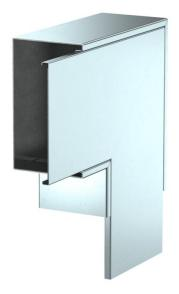
Flat angle with intumescent fire protection mesh for PYROLINE® Rapid PLM installation duct. Suitable for direct wall and ceiling mounting, mounting below system floors and on support systems. Tool-free joint mounting with PLM SI joint connector. The cover is snapped on without tools, allowing rapid inspection and retroassignment. The cover overhang allows offset cover mounting for continuous equipotential bonding of the entire duct section.
