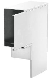
Flat angle with intumescent fire protection mesh for PYROLINE® Rapid PLM installation duct. Suitable for direct wall and ceiling mounting, mounting below system floors and on support systems. Tool-free joint mounting with PLM SI joint connector. The cover is snapped on without tools, allowing rapid inspection and retroassignment. The cover overhang allows offset cover mounting for continuous equipotential bonding of the entire duct section.
