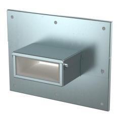
Wall connection collar, 4-sided, with integrated seal for PYROLINE® Rapid PLM installation duct. For mounting in the area of wall and ceiling connections as well as wall penetrations. Can also be used as 3-sided wall connection collar for direct wall or ceiling mounting of the duct.
