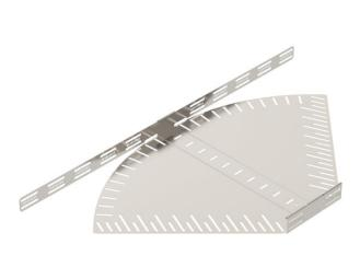
Angle-adjustable bend for the creation of a horizontal branch, fitting for lock and screw-on cable trays of side height 60 mm. Adjustable angle 0–90°. Screwless mounting with double clamps or screw connection with FRS truss-head screws and M6 combination nuts. Can be used indoors and outdoors. Fastening material must be ordered separately.
