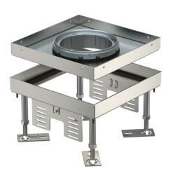
Heavy-duty square cassette for tube body of nominal size 4 for the installation of accessories in trunking systems, raised or cavity floors, in dry or wet-cleaned floors for indoor use. Load class 1 to 10 kN.
