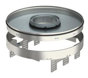
Height-adjustable cassette, decoupled from the floor, of nominal size R9, for tube bodies, for the installation of accessories in dry or wet-cleaned floors for indoor use, for mounting in underfloor boxes UZD350-3, either in conjunction with a mounting lid DUG350-3R9 or UGD350-3R9. Mounting takes place using height adjustment brackets (order separately) in the aluminium frame profile of the underfloor boxes.
