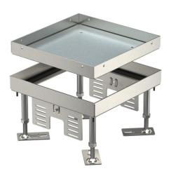
Heavy-duty "blank" square cassette of nominal size 4 for the creation of an inspection opening in trunking systems, raised or cavity floors, in dry or wet-cleaned floors for indoor use. Load class 1 to 10 kN. Only suitable for smooth floor coverings.
