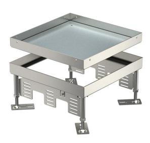
Heavy-duty "blank" square cassette of nominal size 9 for the creation of an inspection opening in trunking systems, raised or cavity floors, in dry or wet-cleaned floors for indoor use. Load class 1 to 10 kN. Only suitable for smooth floor coverings.
