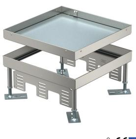
"Blank" height-adjustable cassette for the creation of an inspection opening of nominal size 4. Installation of devices in duct systems, raised and cavity floors in interior dry or wet-care floors. Only suitable for smooth floor coverings. For the installation of three UT4 universal supports for nine single devices with support ring/support clamp or 12 Modul 45® devices. 3 APMT5 cover plates can be installed.
