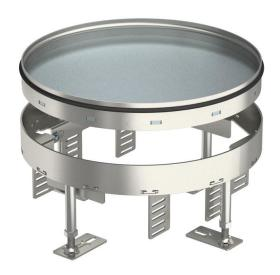
Round, "blank", heavy-duty cassette of nominal size R7 for the creation of an inspection opening in trunking systems, raised and cavity floors, in dry or wet-cleaned floors for indoor use. Load class 2 to 20 kN. Only suitable for smooth floor coverings.
