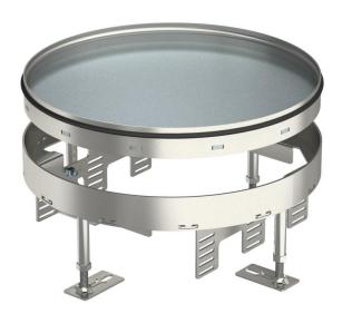
Round, "blank", heavy-duty cassette of nominal size R9 for the creation of an inspection opening in trunking systems, raised and cavity floors, in dry or wet-cleaned floors for indoor use. Load class 2 to 20 kN. Only suitable for smooth floor coverings.
