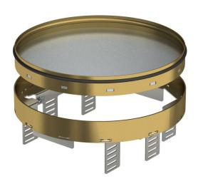
Height-adjustable "blank" cassette, decoupled from the floor, for the creation of an inspection opening of nominal size R7 in dry or wet-cleaned floors for indoor use, for mounting in underfloor boxes UZD350-3, either in conjunction with a blanking lid DUG350-3R7 or in UGD250-3R7. Mounting takes place using levelling profiles (order separately) in the aluminium frame profile of the underfloor boxes. Only suitable for smooth floor coverings.
