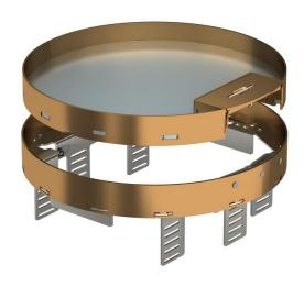
Height-adjustable cassette, decoupled from the floor, of nominal size R7, with cord outlet, for the installation of accessories in dry-cleaned floors for indoor use, for mounting in underfloor boxes UZD350-3, either in conjunction with a mounting lid DUG350-3R7 or UGD350-3R7. Mounting takes place using height adjustment brackets (order separately) in the aluminium frame profile of the underfloor boxes.
