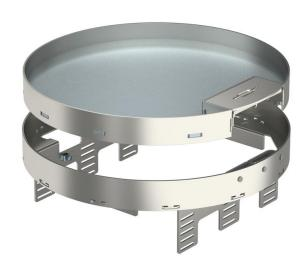
Height-adjustable cassette, decoupled from the floor, of nominal size R9, with cord outlet, for the installation of accessories in dry-cleaned floors for indoor use, for mounting in underfloor boxes UZD350-3, either in conjunction with a mounting lid DUG350-3R9 or UGD350-3R9. Mounting takes place using height adjustment brackets (order separately) in the aluminium frame profile of the underfloor boxes.
