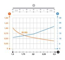
Load diagram, cable tray, type RKS 35
