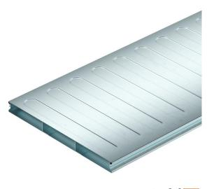
Underfloor duct (2 piece) for routing cables in screed-covered underfloor systems, according to EN 50085-2-2. Removable and continuously lockable duct cover. With separating retainer in the duct base.
