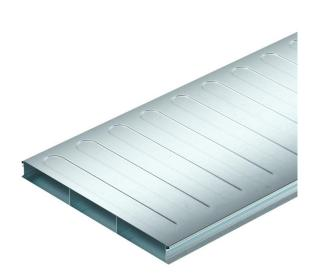
Underfloor duct (2 piece) for routing cables in screed-covered underfloor systems, according to EN 50085-2-2. Removable and continuously lockable duct cover. With separating retainer in the duct base.
