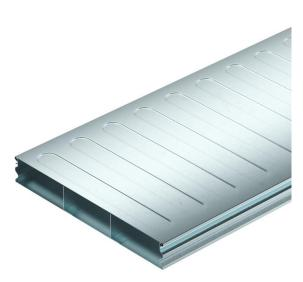
Underfloor duct (2 piece) for routing cables in screed-covered underfloor systems, according to EN 50085-2-2. Removable and continuously lockable duct cover. With separating retainer in the duct base.
