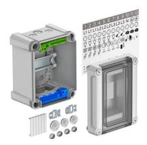
Distribution box with terminal strip for surface mounting, for the current sub-distribution in interior and exterior areas, in accordance with IEC 439-3. With premounted 35 mm hat profile rail. IP66 protection type and IK08 protection rating. Transparent cover to screw on, with cut-out.
