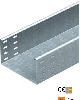
SKS 110 = heavy-duty cable tray system, unperforated, with 110 mm side height. The cable tray has connector perforations on both sides. Straight connectors should be ordered separately and in the appropriate quantity. Magnetic shield insulation without cover 20 dB, with cover 50 dB.
