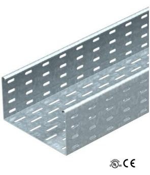
SKS 110 = heavy-duty cable tray system with 110 mm side height. Magnetic shield insulation without cover 20 dB, with cover 50 dB.
