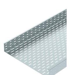
SKS 85 = heavy-duty cable tray system with 85 mm side height. FS version includes connector, type RLVL 85. Magnetic shield insulation without cover 20 dB, with cover 50 dB.
