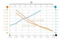
Load diagram, cable ladder, type SLCS 110
