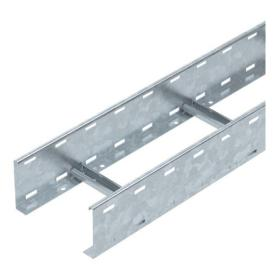
Cable ladder with 110 mm side height with welded C30 profile rungs which are open in an upwards direction. Rolled side rail for reinforcement and as edge protection. Fastening to the bracket takes place using clamps, type LKS 40. The slot dimension of the frame is 16.5 mm and the appropriate U clamp clip is type 2056.
